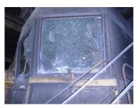
Figure 1: Pulpit Windows Damaged by Explosion
